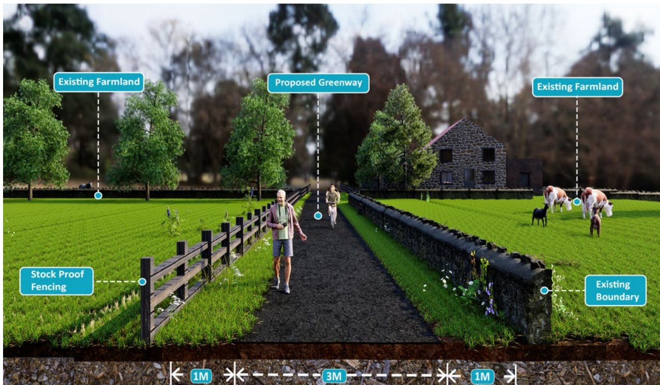
Figure 2.12 Typical Greenway Cross Section Between Farm Boundaries
